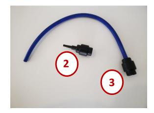
4. The clamp of the provided exhaust sampler might slide and squeeze the silicone hose. Verify that the clamp is over the metal insert that is designed to prevent distortion of the airflow from the exhaust to the sensor.
